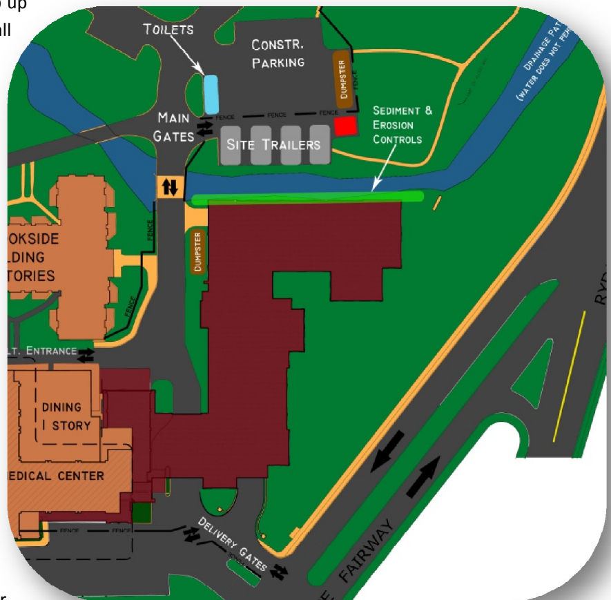
[Figure 03. General Conditions and Temporary Facilities Plan]
